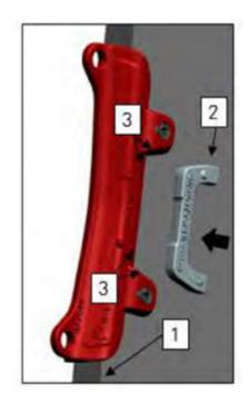
**4.)** Pre-heat the Bucket side to the recommended temperatures and position the weld-on bases (2), until they come into contact with the legs of the Protector (3). Make several tack welds on the back of each base
