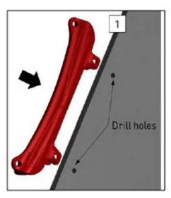
2.) Place Protector on the Bucket side wall, 5-10mm above the adapter wear cap. Ensure Protector is hard against the front of Bucket side (1) and mark the hole centres. Drill holes at 28mm diameter +/- 1mm
