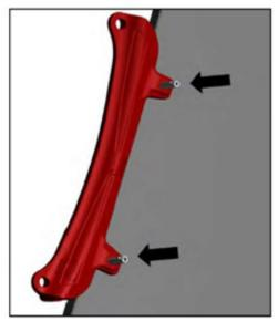
3.) After drilling the holes, insert both pins and turn clockwise until they stop
