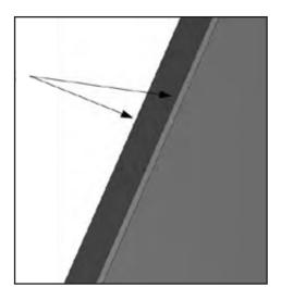
**1.)** Grind a 3mm x 3mm chamfer on both corners of the Bucket side, along the whole length of Protector
